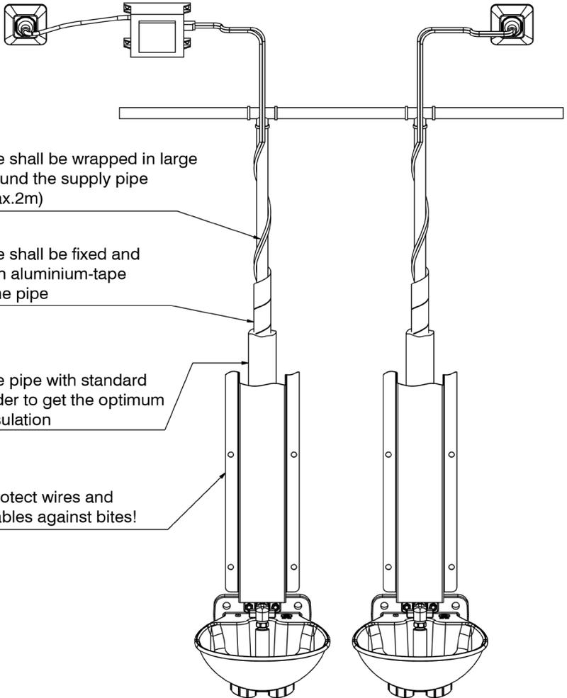
heating cable shall be wrapped in large windings around the supply pipe (min. 1m, max.2m)
